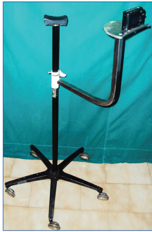
Figure 1: The instrument used for taking consistent photographs
